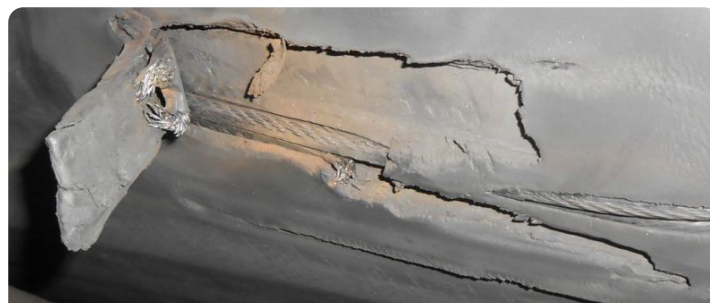
Image depicting a rip in a conveyor belt. Our Safe-T-Rip would detect and activate. Definitions flip side
