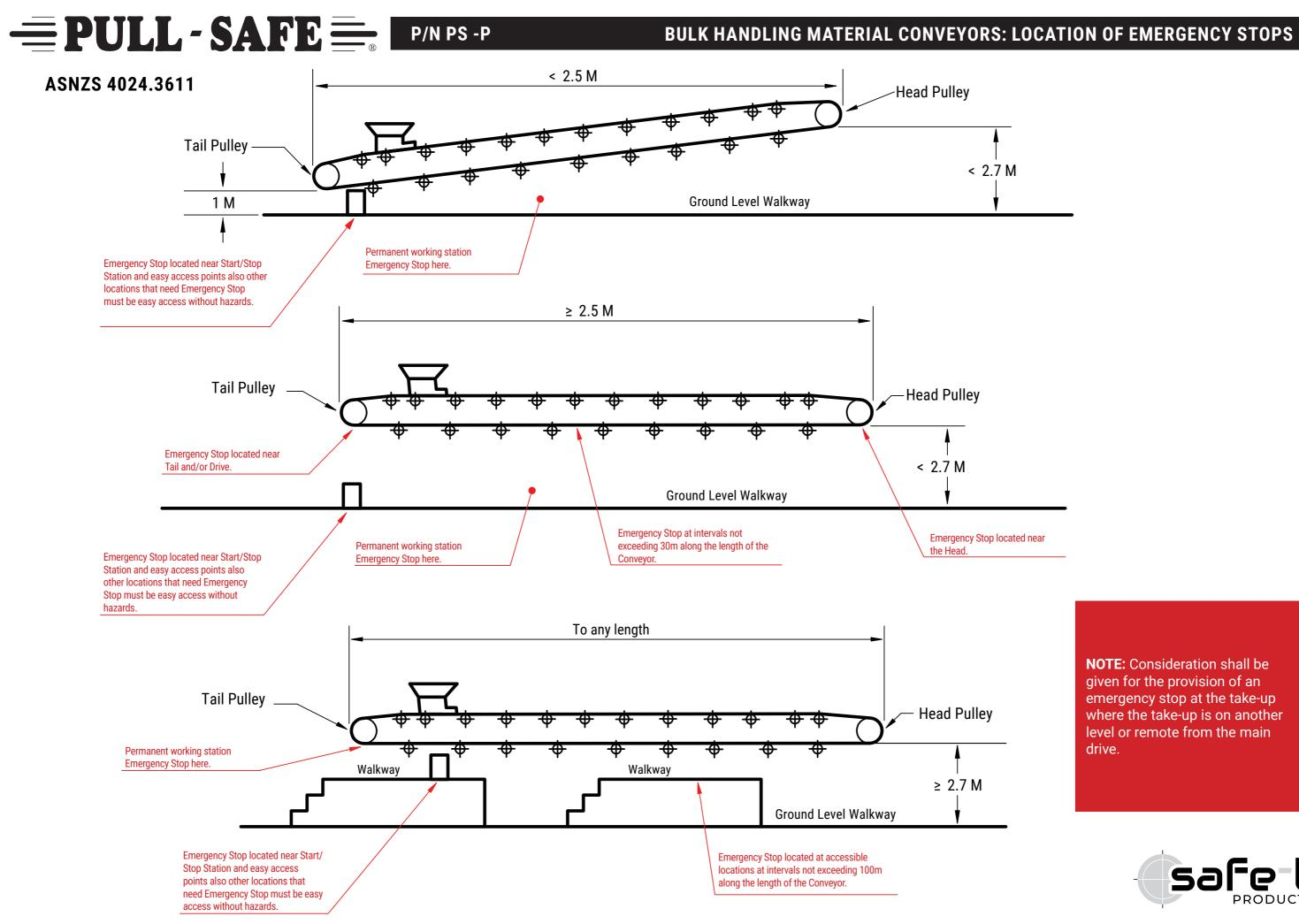
**NOTE:** Consideration shall be given for the provision of an emergency stop at the take-up where the take-up is on another level or remote from the main drive.
