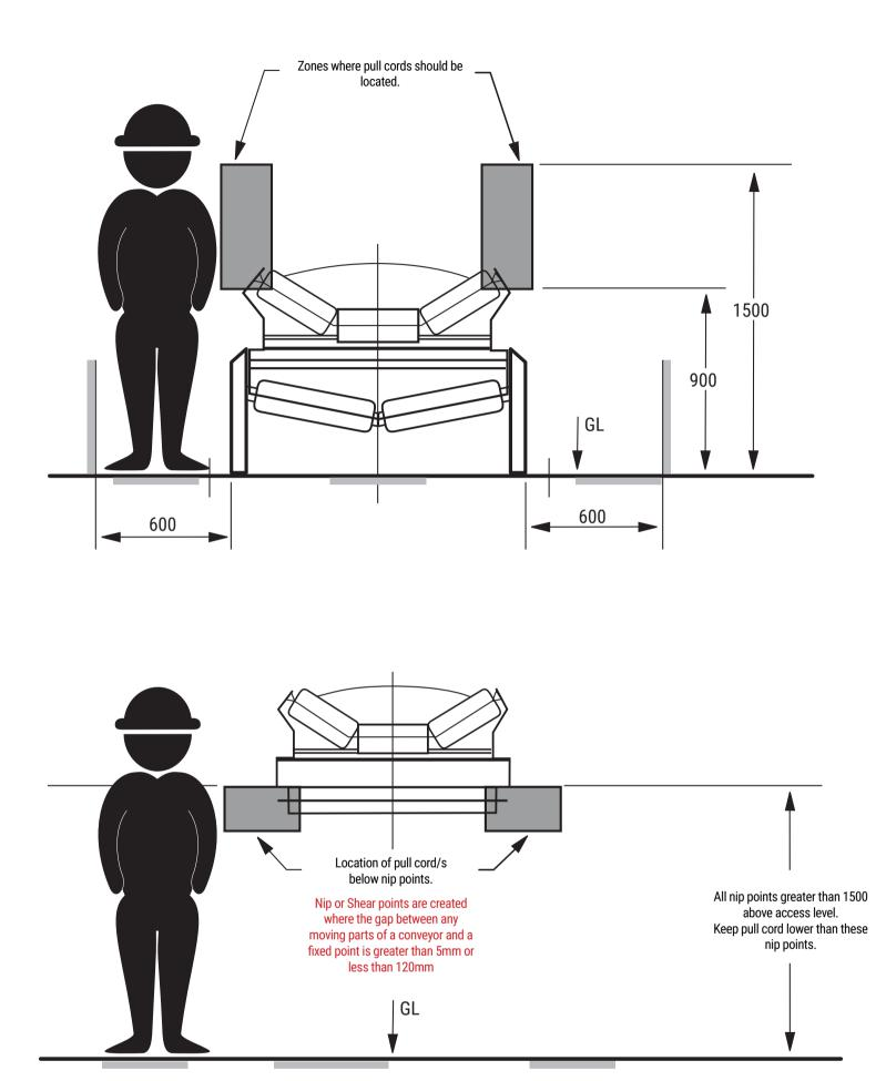
Use STP-NPG Nip Point Gauge to check distances between parts. **NOTE:** Conveyor shall be isolated before task is undertaken.
