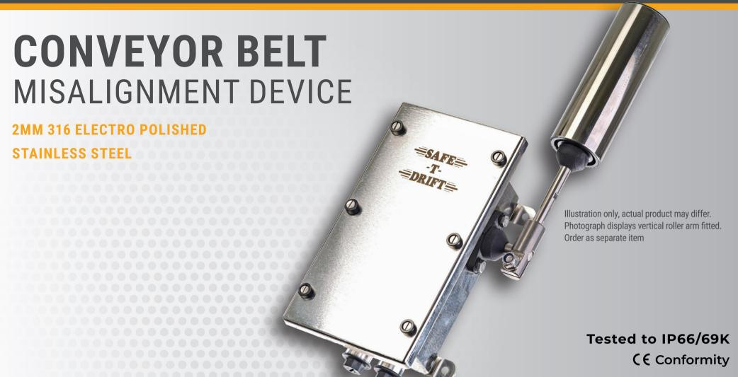
The Safe-T-Drift heavy duty Protective Stop Control Belt Misalignment Device, is made for applications requiring a unit which caters for high speed belt applications, having a cam driven drift alarm micro switch with direct opening action and direct opening action trip micro switch. The cams are individually adjustable for finer alarm and trip points.
