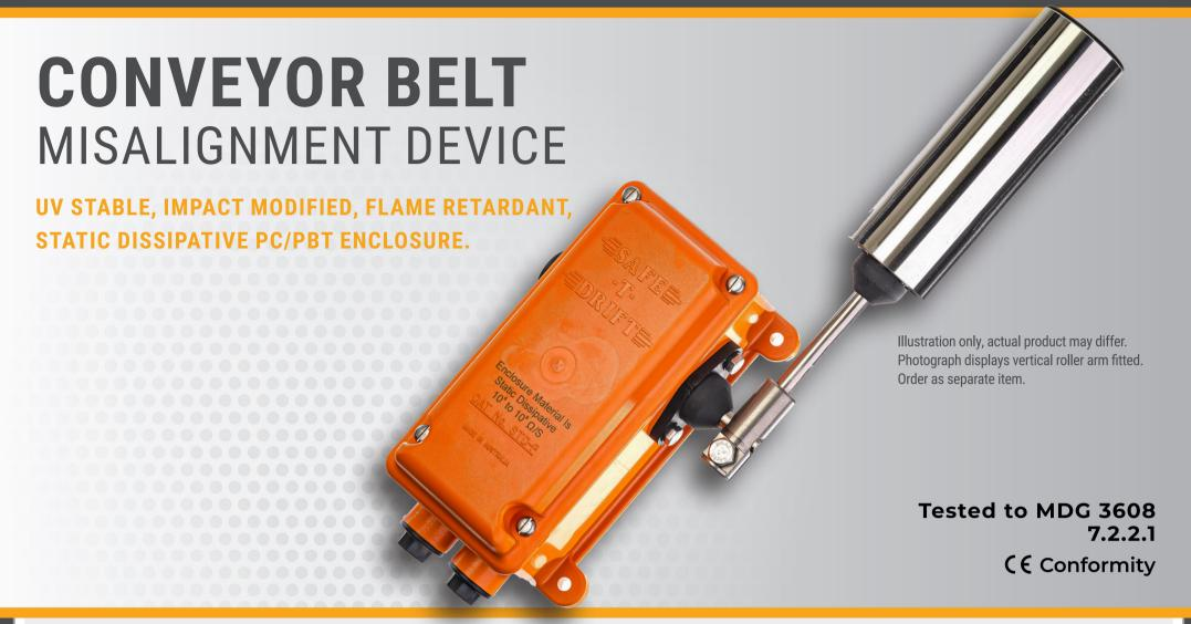
The Safe-T-Drift Ex Static Dissipative heavy duty Protective Stop Control Belt Misalignment Device, is made for applications requiring a unit which caters for high speed belt applications in Ex zones, having a cam driven drift alarm micro switch with direct opening action and direct opening action trip micro switch. The cams are individually adjustable for finer alarm and trip points.
