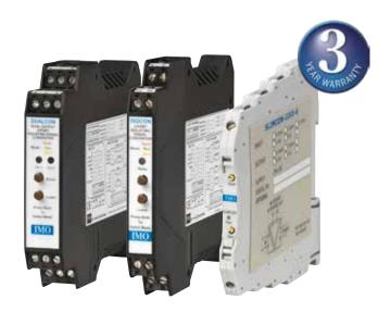
IMO's Signal Conditioners accept a wide range of inputs including 4-20mA, thermocouple, frequency, RTD temperature sensor and voltage signals, which they convert into a high level isolated DC output, or relay switching.
