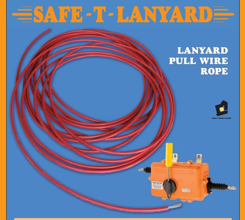
**SAFE-T-LANYARD** Stainless Steel Pull Wire Rope is a UV Stable Red Polyurethane coated 304 Stainless Steel 3mm ID x 5mm OD 6 x 19 construction wire rope, designed and manufactured for the purpose of a lanyard emergency stop pull wire system.
