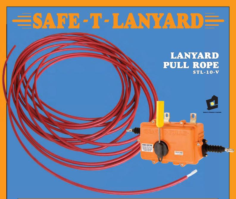
$\blacksquare$ SAFE-T-LANYARD  $\blacksquare$  Vectran  $\blacksquare$  is a UV Stable Red Polyurethane coated LCP (Liquid Crystal Polymer) 3mm ID x 5mm OD multifilament melt spun yarn rope, designed and manufactured for the purpose of a lanyard emergency stop pull wire system.
