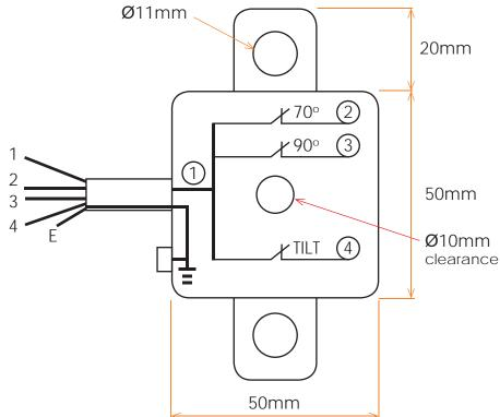
Thermo tilt has as standard three individual switching outputs allowing the installer to know what fault has occurred (whether over temperature, tilt or a combination of both) and then decide what action needs to be taken. Alternative Switching arrangements available on request.
