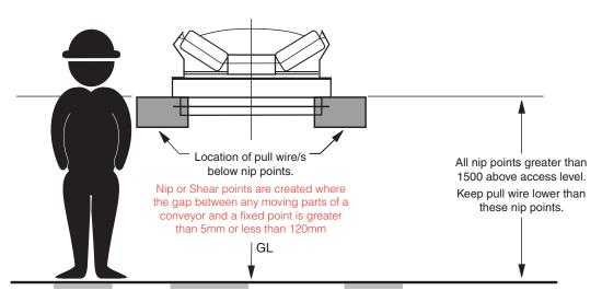
Use STP-NPG Nip Point Gauge to check distances between parts. Note: Conveyor shall be isolated before task is undertaken.
