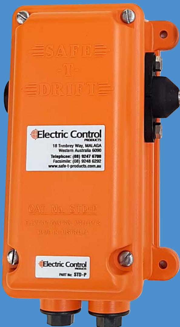
The **SAFE-T-DRIFT** heavy duty Protective Stop Control Belt Misalignment Switch, is made for applications requiring a unit which caters for high speed belt applications, having a cam driven drift alarm micro switch with direct opening action and direct opening action trip micro switch. The cams are individually adjustable for finer alarm and trip points.
