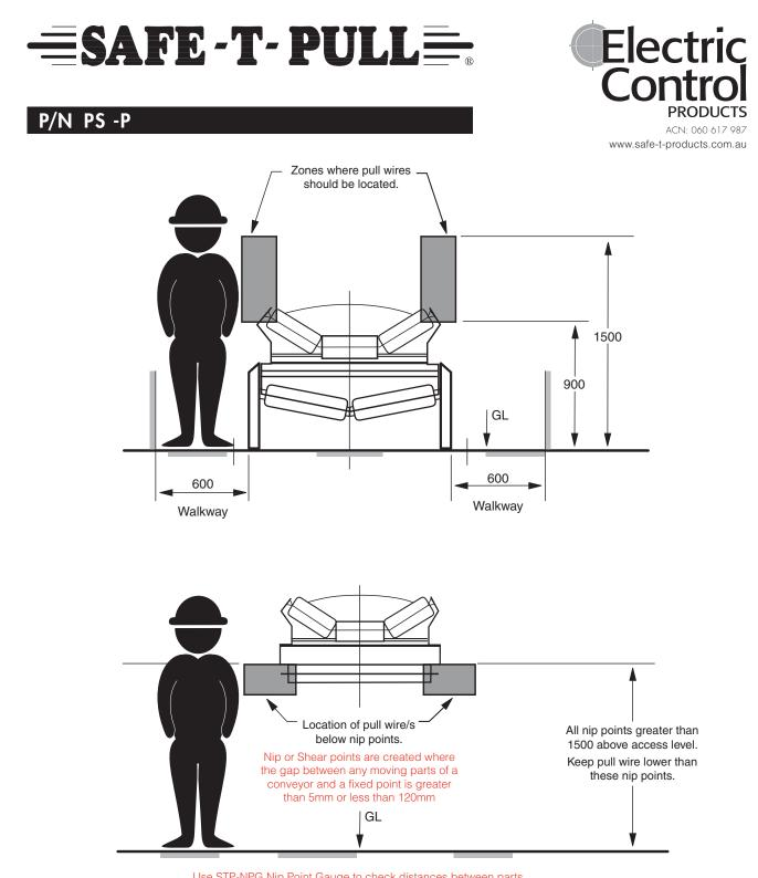
Use STP-NPG Nip Point Gauge to check distances between parts. Note: Conveyor shall be isolated before task is undertaken.
